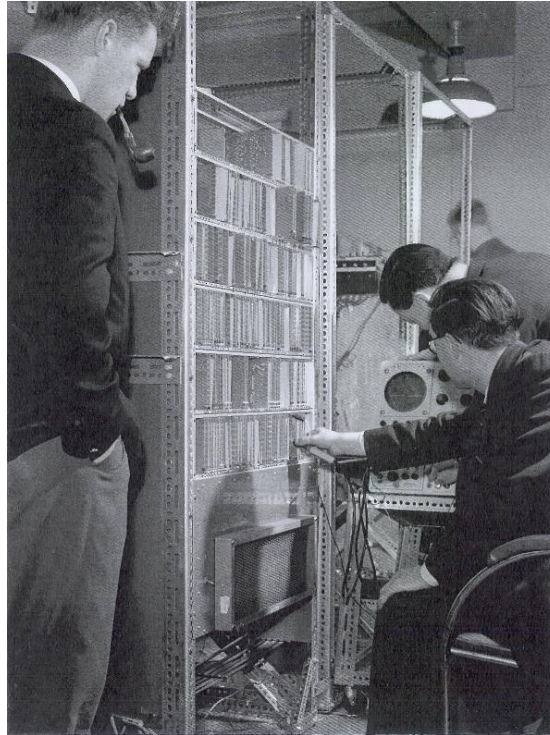
A section of the Pilot Atlas, with boxes attached to a Dexion frame and Gordon Haley, Ianto Warburton and Yao Chen working on the central processor.
